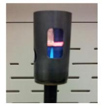
McCampbell Analytical offers a set of comparative standards for the halide flame test used for the determination of chlorinated compounds in refrigeration gas. Refrigeration field technicians can now compare field results to a ref-
